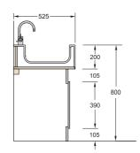
Maximum single Solid Surface washtrough length is 3000mm. Any stud framework is by site.
