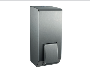
Liquid soap dispenser Stainless steel Wall mounted stainless steel liquid soap dispenser with brushed satin finish, key lock and 900ml refillable reservoir. H251 x W108 x D91mm Code: 0302525
