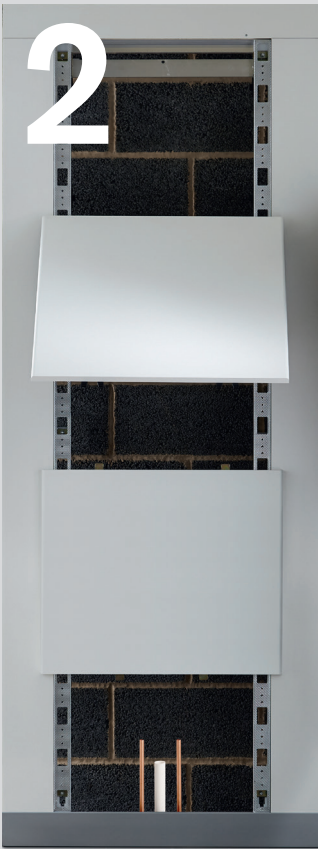
02 Click-fix the first Frameduct unit onto the frame and slide into position. Open the mid panel to a fully hinged position. Attach a vertical flashgap to the frame on either side of the unit, screw-fixing to the frame from the face. Fix tie back to the wall. Repeat until all units are in place.
